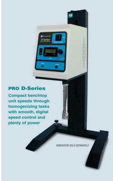
The PRO400 speeds through the homogenization of difficult samples. Shown here with the 02-37000 stainless steel deflector head (see page 8) attached to a 37mm generator for enhanced sample motion.
